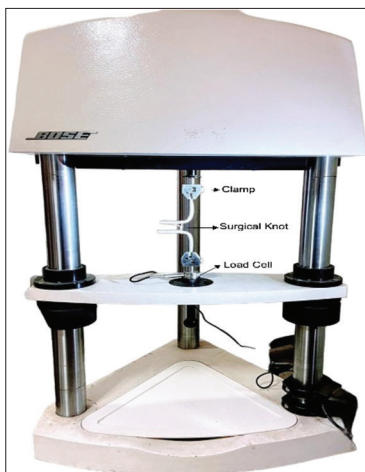
Figure 2: Bose electro force 3200 testing machine showing testing of the knot
